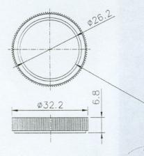
0.5 The Thread of Nut and Housing spec. are the same . Thread Pitch: 1.0mm, Thread depth: 0.5mm.
