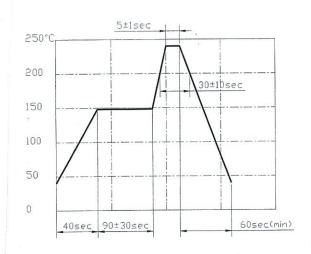
(NOTE: WHEN APPLY 2nd CYCLE OF IR REFLOW PROCESS, THE TRANSDUCER SHOULD BE EXPOSED IN THE ROOM TEMPERATURE AFTER 1st CYCLE OF IR REFLOW PROCESS.)
